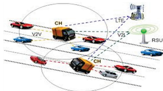
Fig. 1: VANET system architecture
